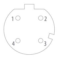
Recommended mating connector type according to IEC 61076-2-10: MM 004-G**x**1-B x) A, C, I, P, R or S-type
