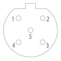
Ethernet connector, M12, female, 4 pins, d-coded, view on rear side of the OPUs A3
